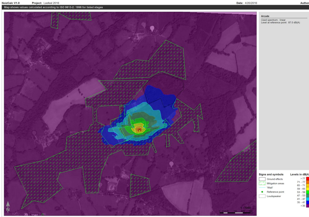
Figure 11: Model Showing Propagation of Noise From Skull Ridge Casino
